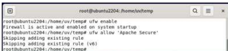
Picture 23 – enabling firewall and creating Apache https rules
