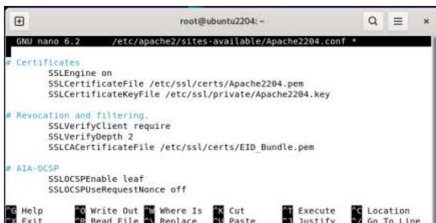
Picture 27 – AIA OCSP configuration is added to SSL section
