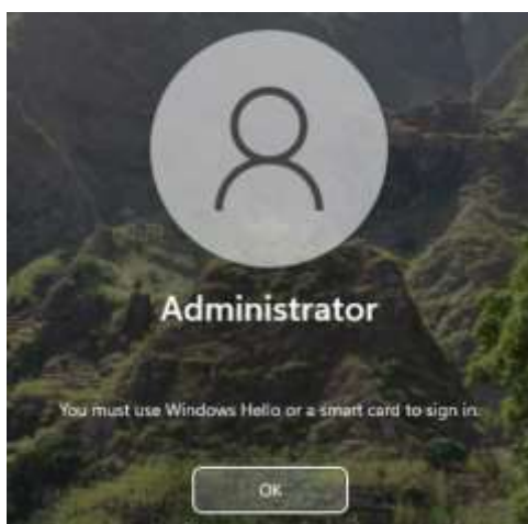
Picture 18 – error message in case user tries to log into domain with username and password, but smart card is required
