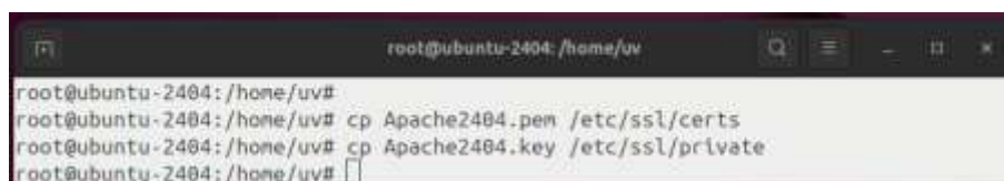
Picture 15 – copying the certificate and its private key to the certificates folder
